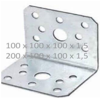
Figure 3 angle brackets. ( to be made according to above design using galvanized sheet metal 1.5mm)
