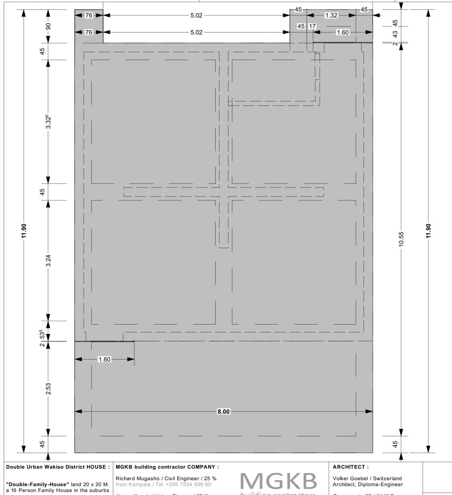
91 sqm concrete foundation plate thickness 10-20 cm with steel mats inside
