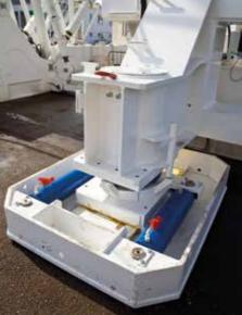
Based on a comprehensive safety concept, the rig has an integrated horizontal-to-vertical pipe handler that can handle a broad range of tubulars including casings up to 4.5 metric tons (5.0 short tons). Together with further automated equipment such as iron roughneck, hydraulic elevator and power slip or slip lifter, tubular handling can be realized hands-off. The whole pipe handling process is controlled from the driller's cabin via a PLC control system with integrated anti-collision system.
