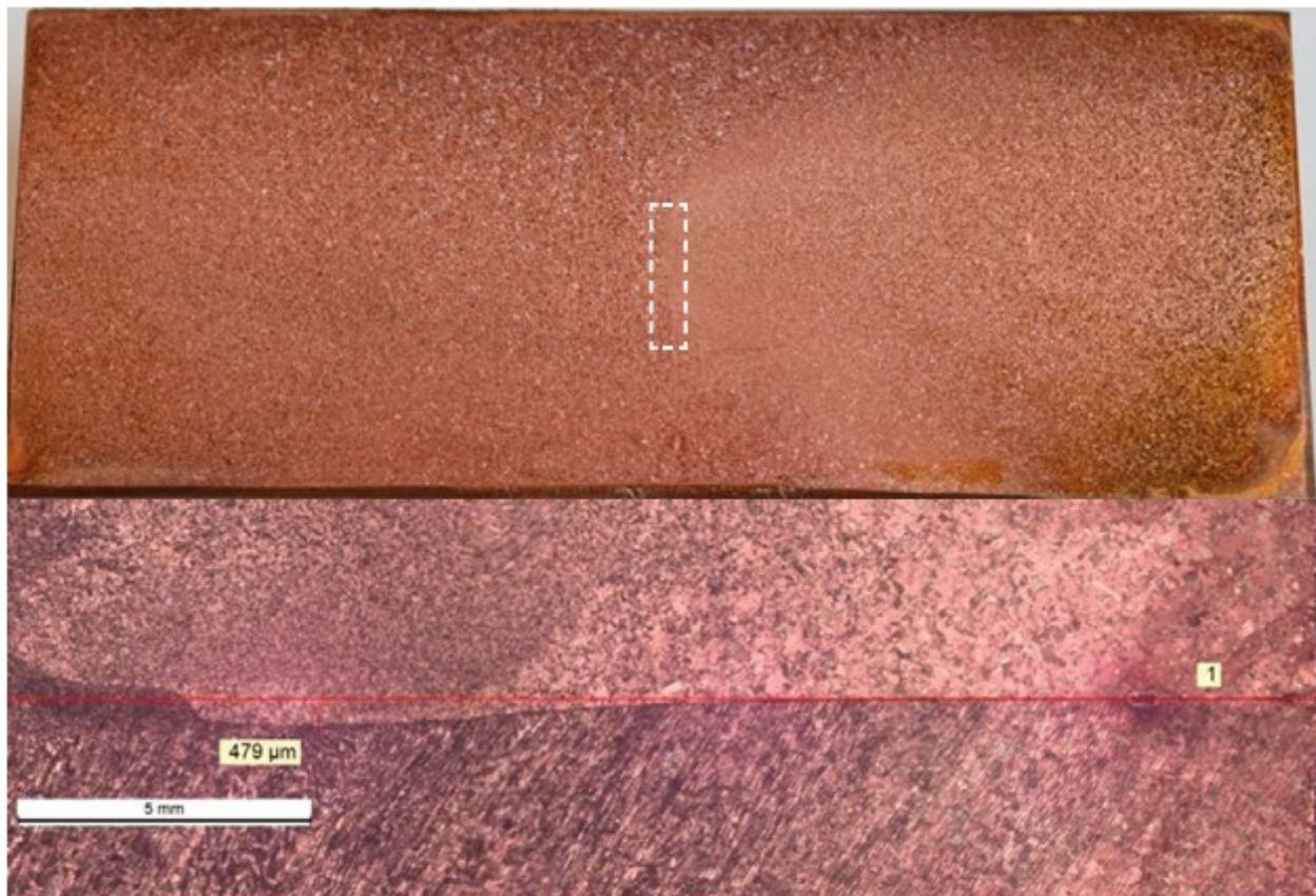
Figure 5-10. Macro sample from weld 604. The top picture shows the weld zone on the right hand side, while the bottom picture shows a zoom of the white dashed box (rotated 90° counter clockwise). A maximum depression of the vertical joint line of 0.479 mm was measured.
