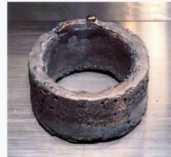
A sample of plutonium metal, shaped like a ring to prevent nuclear criticality
